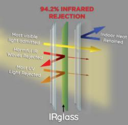
IRglass is energy saving laminated safety glass. Heat is generated by INFRARED.
